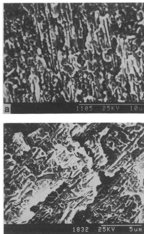
Figure 10 SEM micrographs of 10% LCP/PES blends extruded at 340°C after residence at quiescence within the die for (a) 10 s and (b) 60 s
